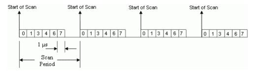
Figure 7. Analog channel scan of voltage inputs example
